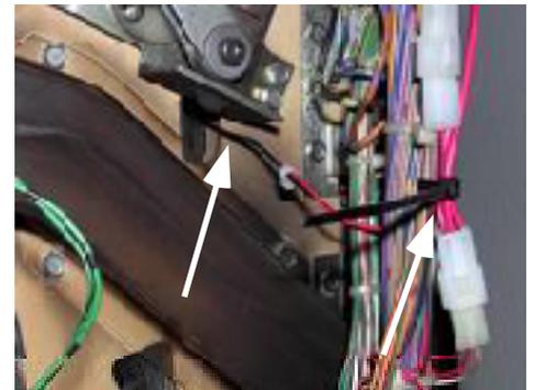
Locate the red and black pair of wires coming from a flash lamp just above (down with the playfield up) the rocket kicker. It is attached under a blue plastic. The wires have a two pin plug on them. Disconnect the two pin plug and carefully connect the rocket connectors to the disconnected connectors. Ty-wrap the rocket wire to the bundle to secure the connectors and wiring.
