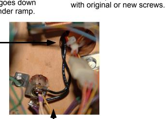
Solder wires to the general illumination lamp or use the alligator leads and wire nuts to attach to the wires and clip on to the lamp socket
