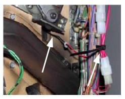
Locate the red and black pair of wires coming from a flash lamp just above (down with the playfield up) the rocket kicker. It is attached under a blue plastic. The wires have a two pin plug on them. Disconnect the two pin plug and carefully connect the rocket connectors to the disconnected connectors. Tywrap the rocket wire to the bundle to secure the connectors and wiring.
