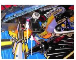
Put the ball guide back and feed the wire behind it. Re-install the rocket plastic with the new rocket plastic on top. Adjust the ball guide and route the wire so it stays behind the guide and up out of the way of the ball. The wire should enter the right side of the hole so the kicker won't hit it. See the next picture too.
