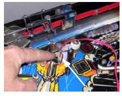
Bring the playfield down to the rests and remove the plastic and ball guide. The rocket is mounted to its own plastic that will be installed over the rocket plastic. Feed the wire plugs through the kicker hole holding the kicker to the left with a finger. Feed nearly all the wire through the hole.
