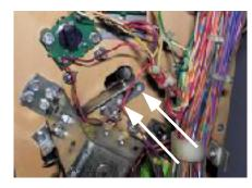
Raise the playfield to the full vertical position. Take care not to have the balls fall and damage anything. Remove two screws from the right end of rocket ball kicker bracket and rotate the kicker clockwise down.
