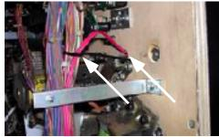
Raise the playfield to the full vertical position again. Re-install the two rocket ball kicker screws. Ty-wrap the the wire from the rocket to the bundle as in the picture and adjust it so the wire stays against the upper side of the hole and away from the kicker arm.
