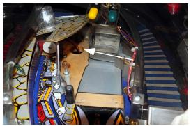
Remove the 8mm nut from the tip of the plastic next to the train target. Also remove the ball ramp to the right by removing two screws as indicated at the entrance to the ramp. locate the hole in the playfield under the plastic and see the wire that comes from the flasher going through it. Install the train's cable connector and cable through this hole.
